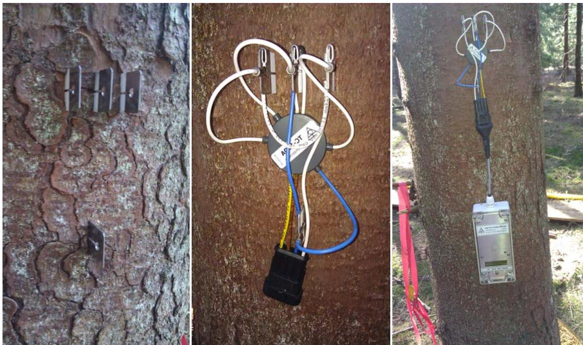
Figure 3: EMS 51 system, first part showing the inserted steel electrodes inserted in tree trunk, second part showing the heated and unheated needles inserted in the electrodes, third part showing the measurement module connected to the needles and electrodes. (Photo by: Anke Hartmanns)
